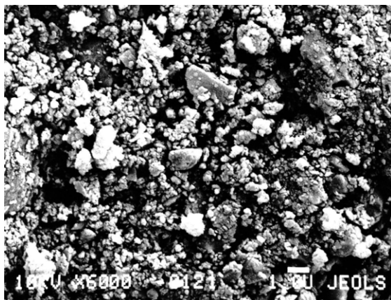
Fig. 6. Micrograph of the surface of the initial shungite-III (Magnification 6 000).
